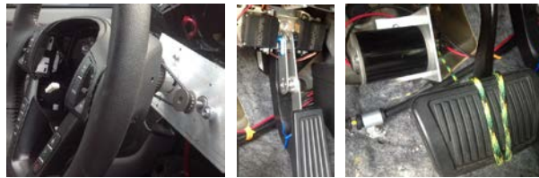
Fig. 7. Motor and servo controlled actuation of steering (left), acceleration (center), and braking (right) to enable drive-by-wire control of a KIA Optima.
