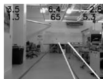
Fig. 4. Case where a spurious lane boundary (white) is rejected – the trusted line (gray) is used to predict the location of the rejected lane boundary (off-white) using the perspective transform.
