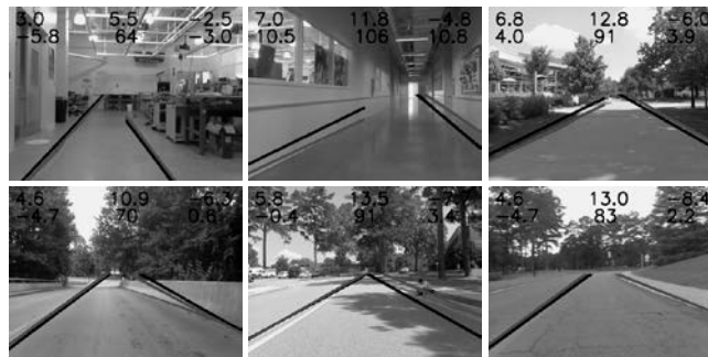
Fig. 3. Various scenes successfully navigated by the vehicle including a 5 ft wide artificial lane in a laboratory setting, hallway, sidewalk, and several different road conditions.
