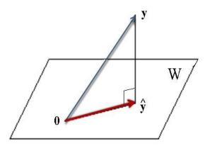
Figure: Illustration of an orthogonal projection. Note that  $dist(\mathbf{y}, \hat{\mathbf{y}})$  is the shortest distance between  $\mathbf{y}$  and the points on W.
