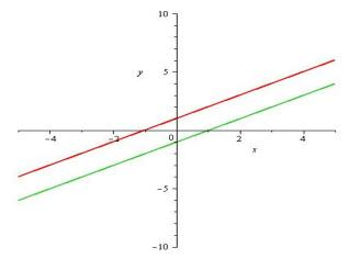
Figure: The system x - y = -1 and 2x - 2y = 2 with solution set  $\emptyset$ . These equations represent parallel lines having no common points.
