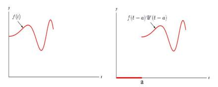
Figure: The function  $f(t-a)\mathcal{U}(t-a)$  has the graph of f shifted a units to the right with value of zero for t to the left of a.
