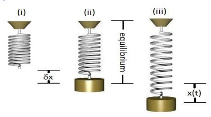
Figure: The displacement in equilibrium  $\delta x$  is the difference between spring only length, and spring-mass equilibrium length.
