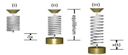
Figure: (i) Spring only *equilibrium*. (ii) Spring-mass system **equilibrium**. The difference  $\delta x$  will be called *displacement in equilibrium*. Our variable x(t) will be displacement of the Spring-Mass system.
