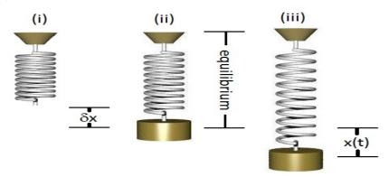
Figure: (i) Spring only *equilibrium*. (ii) Spring-mass system **equilibrium**. The difference  $\delta x$  will be called *displacement in equilibrium*. Our variable x(t) will be displacement of the Spring-Mass system.
