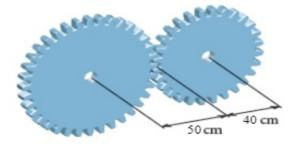
Points on the rims of the gears share a common linear velocity  $\nu$ . If we call the radius and angular velocity of the smaller gear  $r_1$  and  $\omega_1$  and the radius and angular velocity of the larger gear  $r_2$  and  $\omega_2$ , we have
