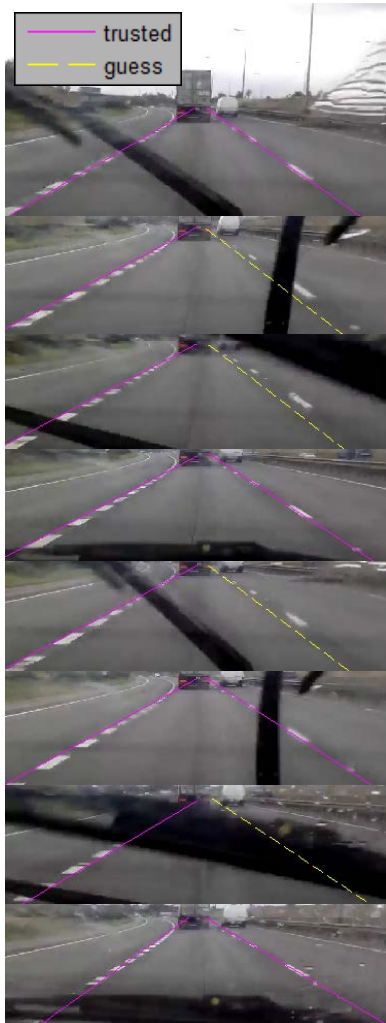
Figure 8: Successful lane boundary detection while raining.
