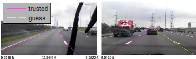
Figure 6: Road images where a) both detected lane boundaries are trusted and b) where one boundary is trusted and the other is approximated.
