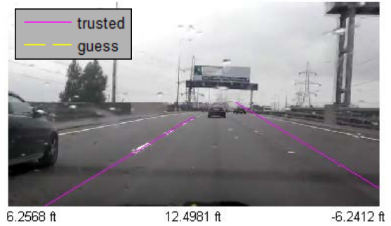
Figure 9: Example of outcome 2) where both detected boundary lines are trusted but one (the left) is correct while the other (the right) is slightly off.
