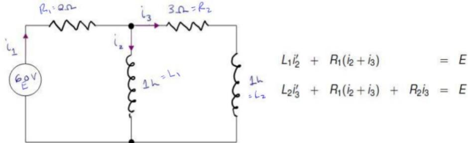
**Figure:** If we label current  $i_2$  as  $x(t)$  and current  $i_3$  as  $y(t)$ , we get the system of equations below. (Assuming  $i_1(0) = 0$ .)
