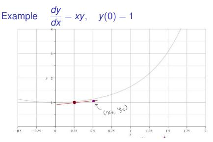
Figure: We go out *h* more units to  $x_2 = x_1 + h$ . Pick the point on the tangent line  $(x_2, y_2)$ , and use this to approximate  $y(x_2)$ . So  $y_2 \approx y(x_2)$
