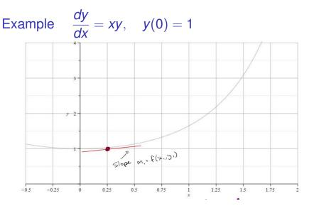
Figure: Now we start with the point  $(x_1, y_1)$  and repeat the process. We get the slope  $m_1 = f(x_1, y_1)$  and draw a tangent line through  $(x_1, y_1)$  with slope  $m_1$ .
