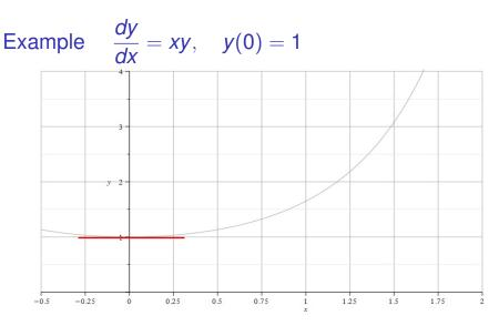
Figure: So we draw a little tangent line (we know the point and slope). Then we increase x, say  $x_1 = x_0 + h$ , and approximate the solution value  $y(x_1)$  with the value on the tangent line  $y_1$ . So  $y_1 \approx y(x_1)$ .
