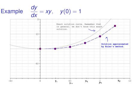
Figure: We can repeat this process at the new point to obtain the next point. We build an approximate solution by advancing the independent variable and connect the points  $(x_0, y_0), (x_1, y_1), \dots, (x_n, y_n)$ .
