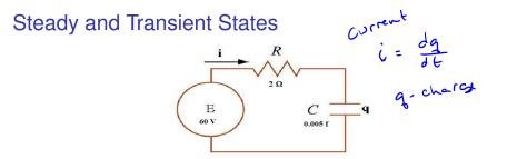
Figure: The charge q(t) on the capacitor in the given curcuit satisfies a first order linear equation.
