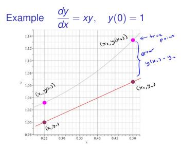
Figure: If we zoom in, we can see that there is some error. But as long as *h* is small, the point on the tangent line approximates the point on the actual solution curve.
