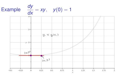
Figure: We take the approximation to the true function *y* at the point  $x_1 = x_0 + h$  to be the point on the tangent line.
