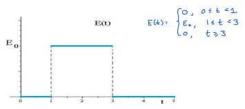
Figure: A switch is closed for two seconds from t = 1 until t = 3 during which a constant  $E_0$  volts is applied.
