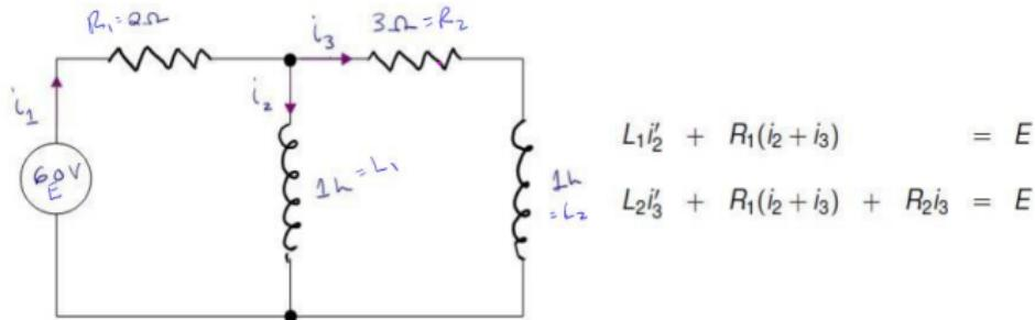
**Figure:** If we label current  $i_2$  as  $x(t)$  and current  $i_3$  as  $y(t)$ , we get the system of equations below. (Assuming  $i_1(0) = 0$ .)
