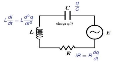
Figure: The potential drop across the capacitor is q/C, across the resistor is *iR*, and across the inductor is  $L_{dt}^{di}$ .
