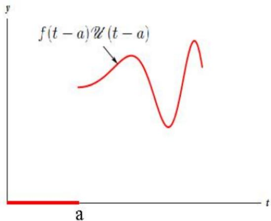
**Figure:** The function  $f(t - a)\mathcal{U}(t - a)$  has the graph of  $f$  shifted  $a$  units to the right with value of zero for  $t$  to the left of  $a$ .
