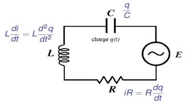
Figure: The potential drop across the capacitor is q/C, across the resistor is iR, and across the inductor is  $L\frac{di}{dt}$ .
