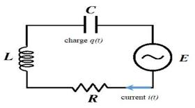
Figure: Simple circuit with inductance L, resistance R, capacitance C, and implied voltage E. The current  $i(t) = \frac{dq}{dt}$  where q is the charge on the capacitor at time t in seconds.
