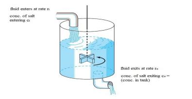
Figure: Values for  $c_i$ ,  $r_i$ , and  $r_o$  are given in the problem statement. The well mixed assumption means that  $c_o$  will match the concentration in the tank.
