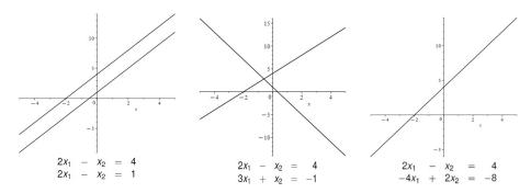
Figure: Lines determined by two linear equations in two variables illustrating the three possible geometric relationships.
