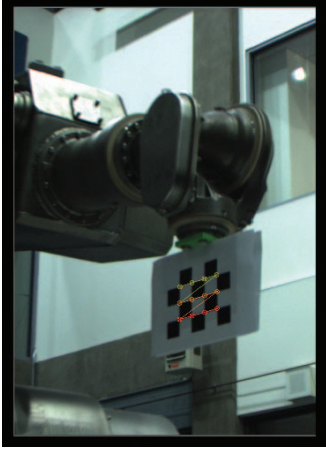
Fig. 1. Image feature extraction: of the twelve checkerboard vertices pictured, the outer four constitute \mathbf{y} (goal coordinates not shown).
